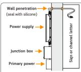
5. Make secondary connections: Ensure all secondary connections are RED-TO-RED and BLACK-TO-BLACK. If wires go through wall - seal with silicone to avoid water damage. Also check and fix with gasket or other rubber material sharp edges because it can damage the wire and there could occur short circuit connections
